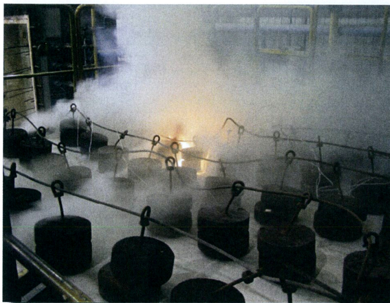
View of the light steel floor under a load of 2.5 kPa at the end of the 90 minutes fire resistance test at BRE.
